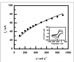
**Fig. 5** Example electrochemical area measurements for a NiCo thin film. The sample had a deposited charge of 1000 mC. The *inset* shows CV measurements in 5 mM Ru(NH<sub>3</sub>)<sub>6</sub>Cl<sub>3</sub> and 1 M KCl at 200, 400, and 800 mV/s. The magnitude of the peak cathodic current,  $I_{pr}$ , is fit to a square root function vs. scan rate, v, to determine the area,  $A_{ecr}$  of the sample using the Randles–Sevcik equation
