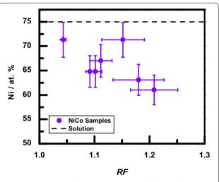
**Fig. 3** Ni composition for the NiCo samples as a function of the average roughness factor, *RF*, of the samples. *Composition error bars* represent the typical EDS uncertainty. The *dashed line* indicates the Ni composition in the deposition solution
